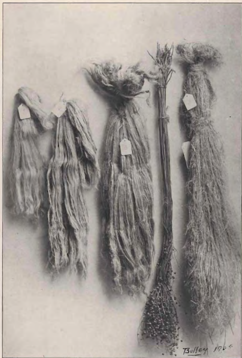
Plate 20. Four types of flax fibre, and a bundle of North Dakota grown Russian fibre flax seeded at the rate of one-half bushel to the acre, showing the coarsest form, 47 inches high. Binder twine type. No. 1, best quality Courtrai made fibre. No. 2, best quality North Russian (Vologda) prepared fibre. No. 3, hand broken and partly scutched at the North Dakota Experiment Station from coarse straw similar to the that shown alongside. No. 4, hand broken and scutched fibre prepared from North Dakota grown dew retted straw.
