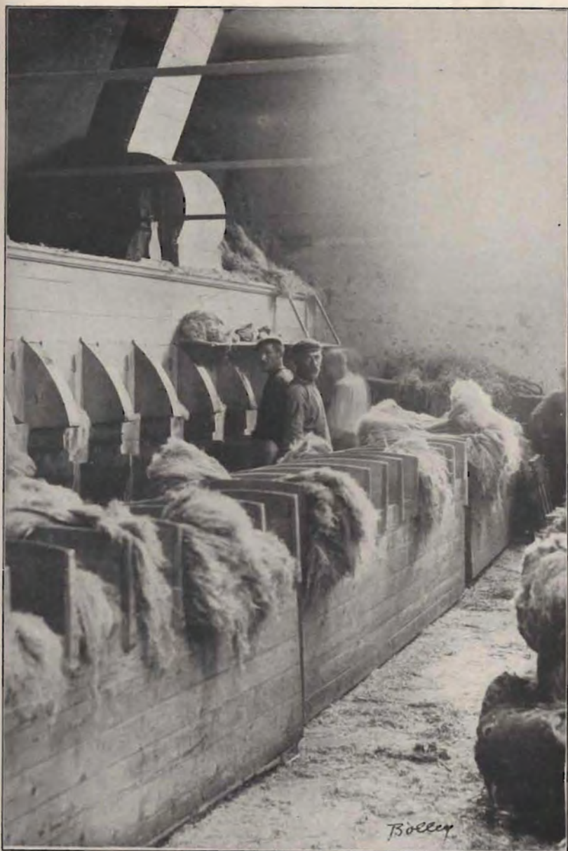
Plate 9. A Belgium scutching mill showing position of the laborer with reference to scutching wheels and the sorting stalls.
