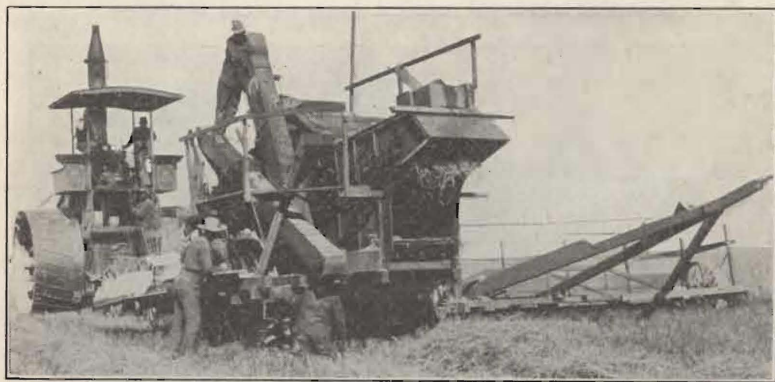
Fig. 25.—Combined Header and Thresher, not commonly used on flax, it is unsatisfactory because of its disease relations and because of difficulty in regulating the speed of the thresher.
