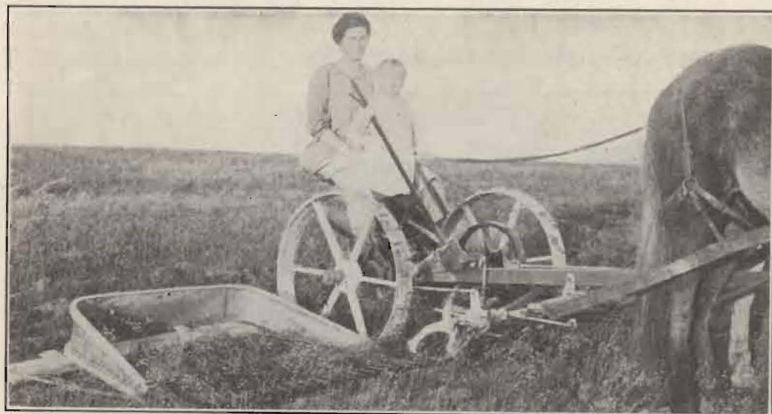
Fig. 24.—The first crop under rough conditions. A buncher attached to the mower is sometimes used on very short flax, but cannot do good work under such ground conditions as here shown.
