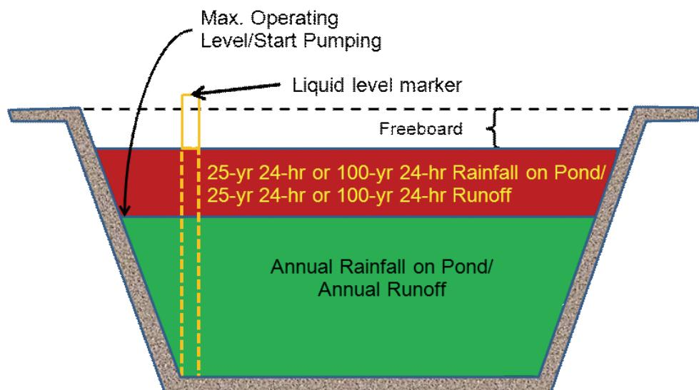
**Fig. 1. Capacity of a runoff storage pond (not to scale).**
