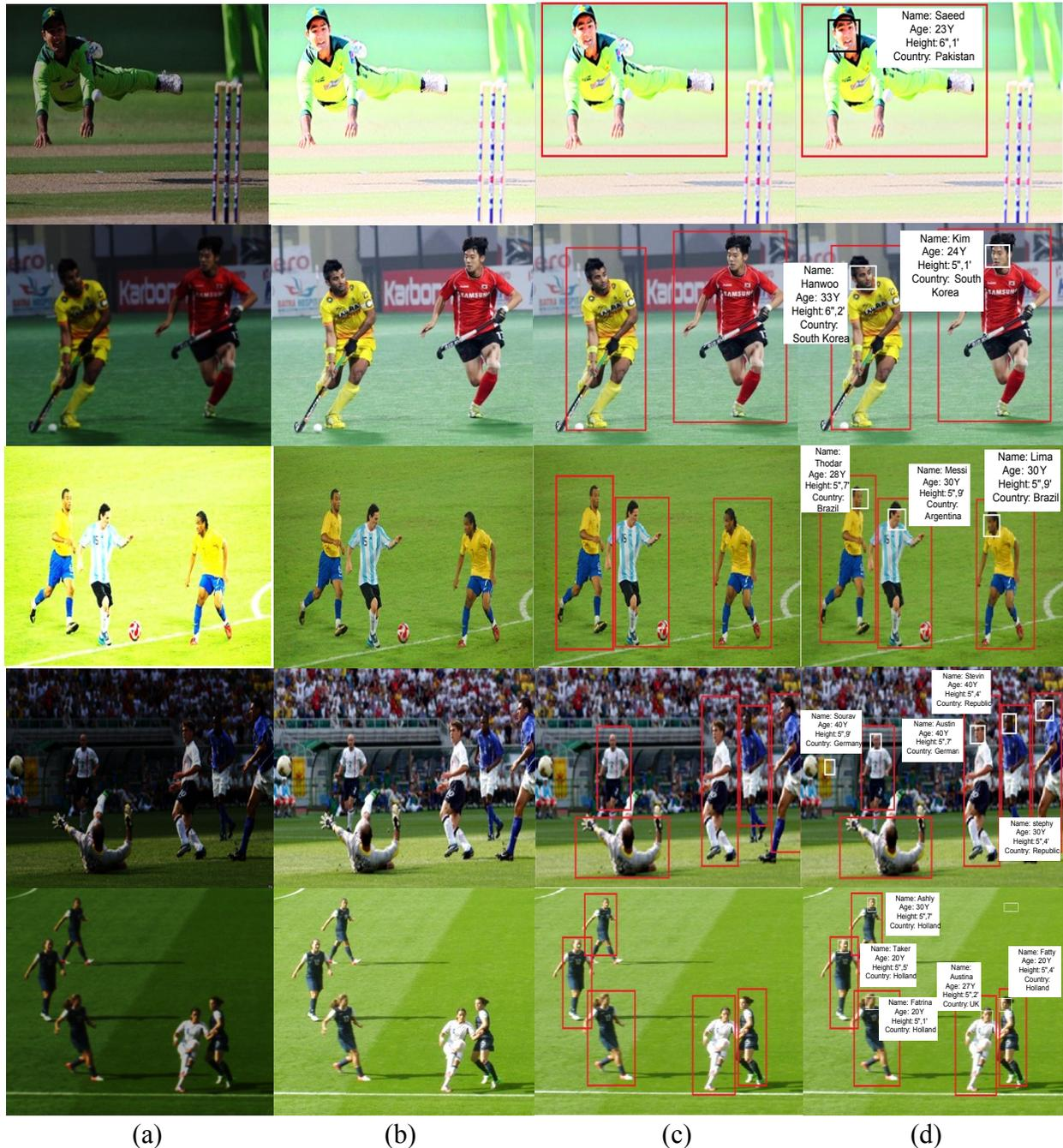
Fig. 5.1. Complete output of the developed EAR system on sample images: (a) original degraded input player images, (b) player image enhancement, (c) player detection, (d) player face recognition and display of statistics.
