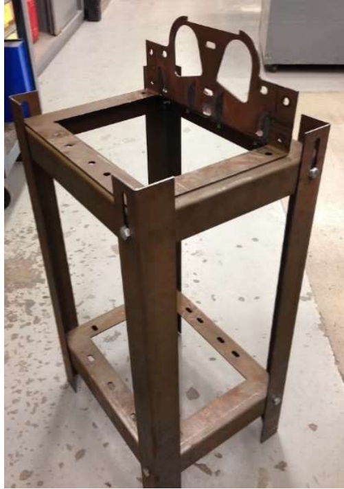
Figure 15. Stand to hold the new seed delivery system.
