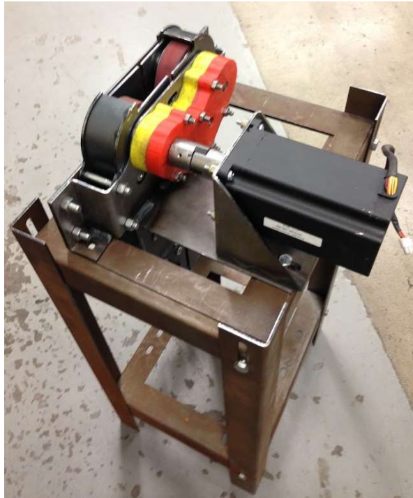
Figure 16. Stand with the new seed delivery system and stepper motor.
