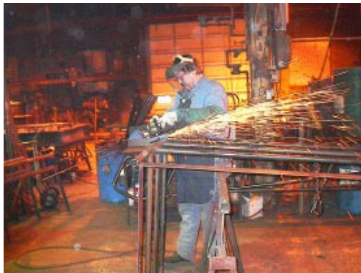
Mid America Steel, Inc. plant (formerly Fargo Foundry). Mike Heger sanding the weld smooth on a metal handrail for a power plant located in Washington state, 2002. (Kenneth Price, Mid America Steel, Inc)
