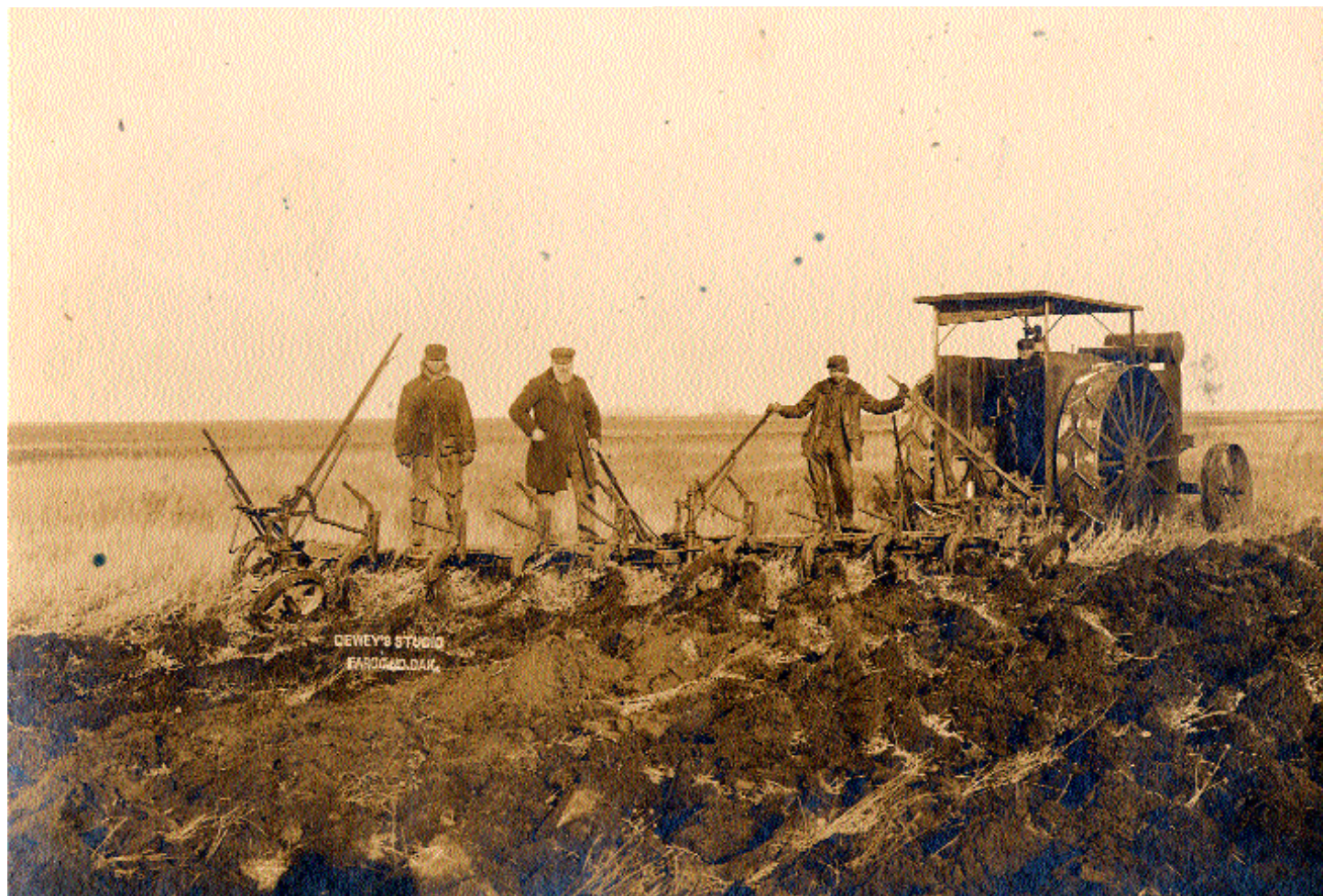
Frank Larson, Henry Larson, William Larson and Albert Boots on a Flour City gas tractor pulling two 4-bottom plows, near Gardner, ND, 1910. (Charlotte Larson Owens, Dewey's Studio)
