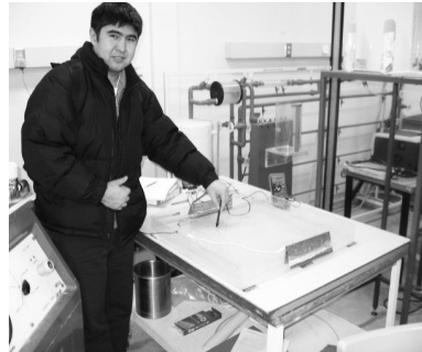
Musayev works on the electrical analogy apparatus in the fluid mechanics laboratory to learn about groundwater flow patterns.
