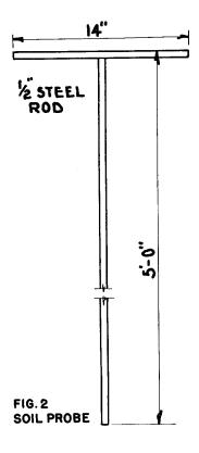
You can tell how deep the soil has been wetted by using a soil probe. This probe can be made by welding a crosspiece on top of a 5-foot length of 1/2-inch steel rod. The probe can be pushed easily into wet soil, but will stop when it hits dry dirt. Stop irrigating when the probe goes down 2/3 of the depth you want to irrigate. Stop irrigating when the probe strikes dry soil at 2 feet for small grains and pasture, 2 feet 8 inches in corn, sugar beets and potatoes, and at 4 feet in alfalfa.
