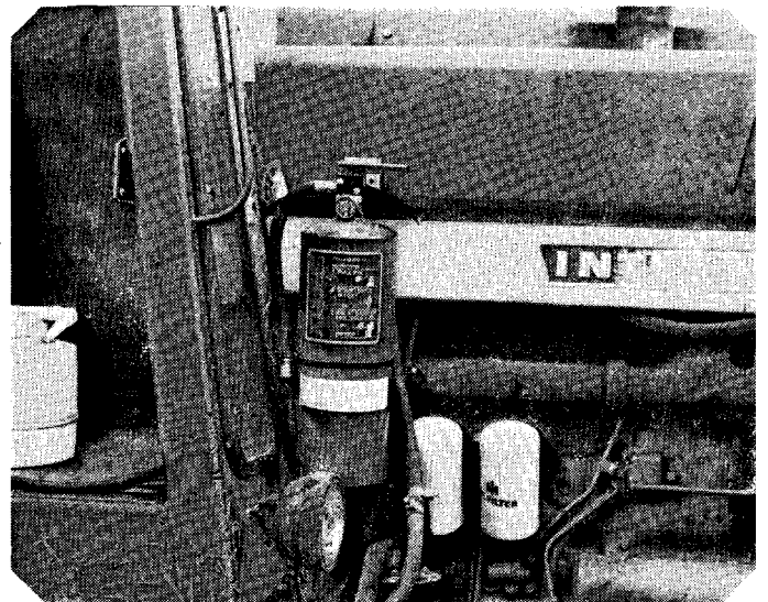
Mount extinguishers on farm implements so they can be reached from the ground or near the operators platform.
