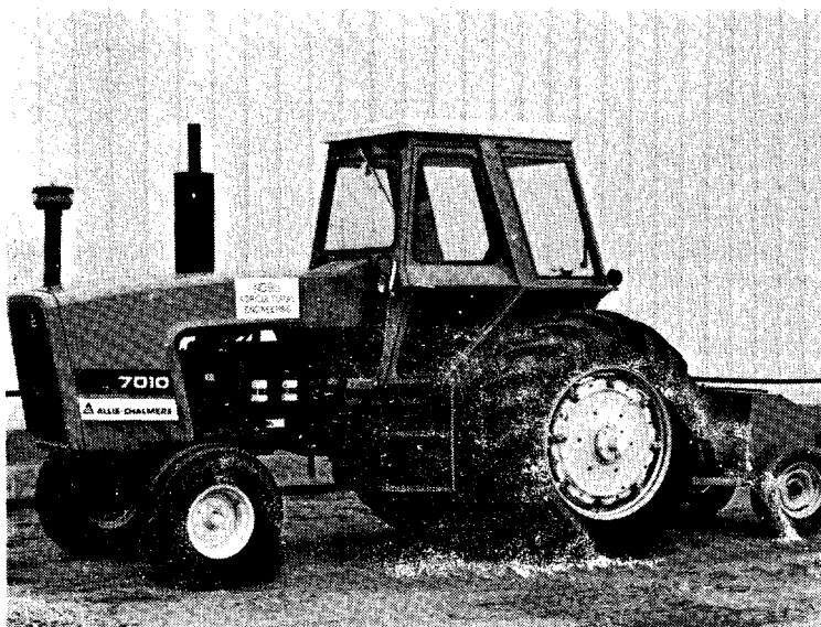
Figure 4. Tractor engine efficiency is determined by measuring the horsepower produced and the gallons of fuel used.
