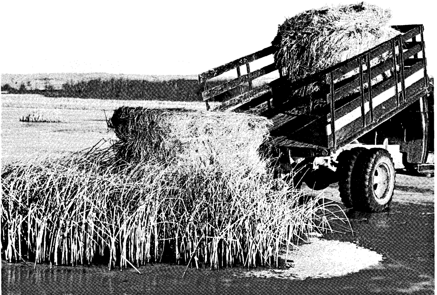
Figure 15. Large round bales may be placed in wetland during the winter using standard farm trucks equipped with hoists. (I. Rostad)
