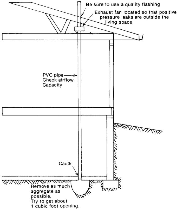
**Figure 6. Depressurization of the soil by applying suction to the aggregate below the slab.**
