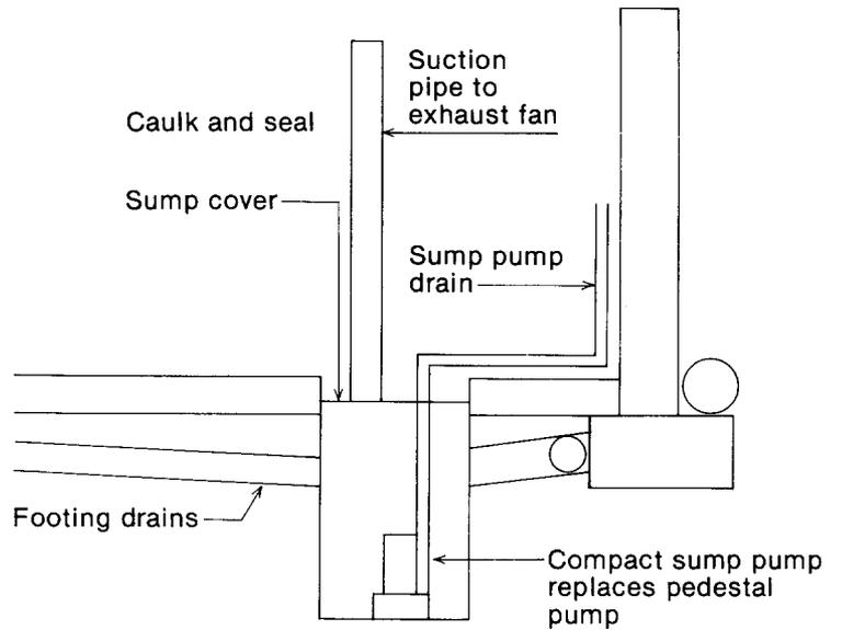
**Figure 8. Converting a sump hole into a radon collection sump. Be sure to caulk all joints between materials.**
