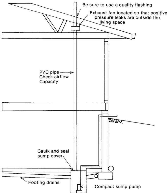
**Figure 7. Soil depressurization by suction on sump hole.**
