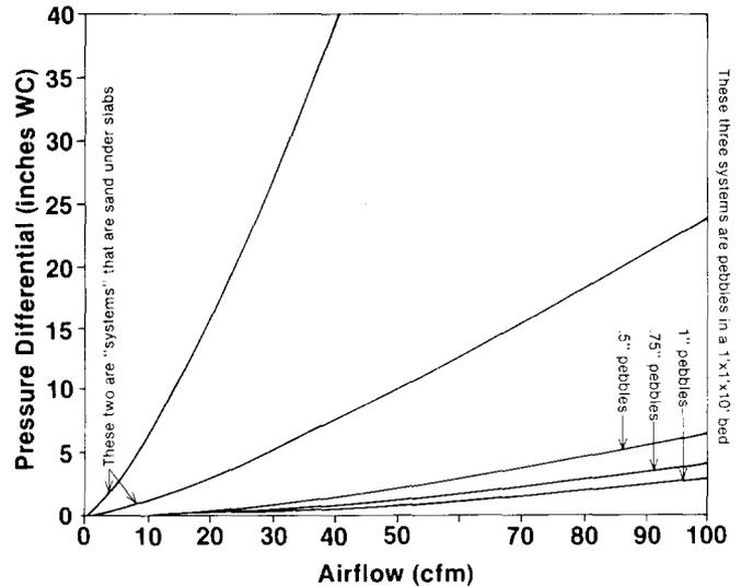
**Figure 10. Pressure vs airflow curves for different aggregates.**
