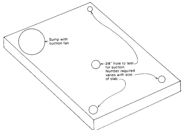
**Figure 9. Place test opening at strategic locations around slab to insure that a suction exists at all locations. Be sure to caulk holes after completing the test.**
