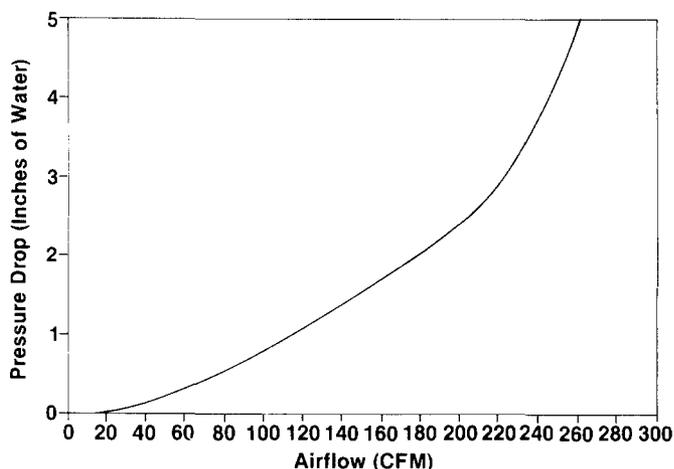
Figure 12. Pressure drop through 100 feet of 4 inch PVC pipe.
