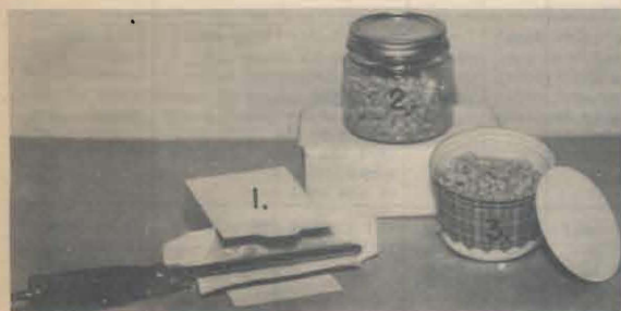
Figure 1. Container for vegetables; (1) End-opening paperboard container with a lining of moisture-proof, vapor-proof, heat-sealing paper; (2) Glass container; (3) Heavily waxed tub type container.
