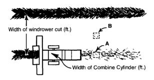
Divide the result of Step 4 by the number of kernels for the particular crop for one bushel per acre loss (Table). This is the approximate machinery loss in bushels per acre.
