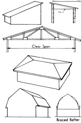
SHED - Roof slopes one direction. Simple to build. Can go up to 20 ft. wide. Wider clearspans are uneconomical and post support used.
