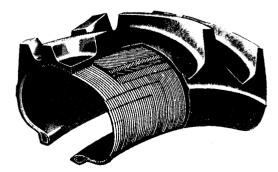
Cords in a radial-ply tire are in parallel layers with belts under the tread area.
