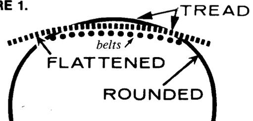
Flattened tread base of the radial-ply tire with encircling belts distributes weight more evenly than conventional rounded base.
