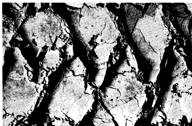
Tire imprint made with 15 percent slippage
