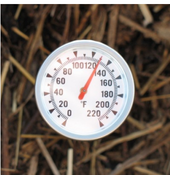
After 24 hours of manure piling, the temperature has reached 130 F.
