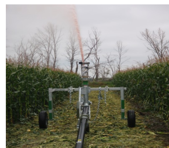
Applying pond effluent with a traveling gun.
