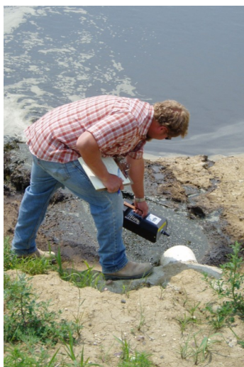
Monitoring hydrogen sulfide emissions from a containment pond.
