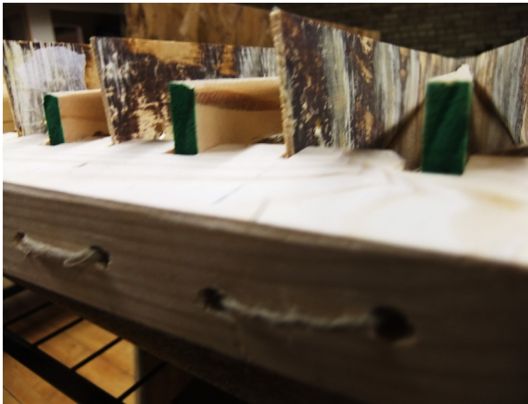
The process that involves stringing together the plywood and pine blades throughout the spine.
