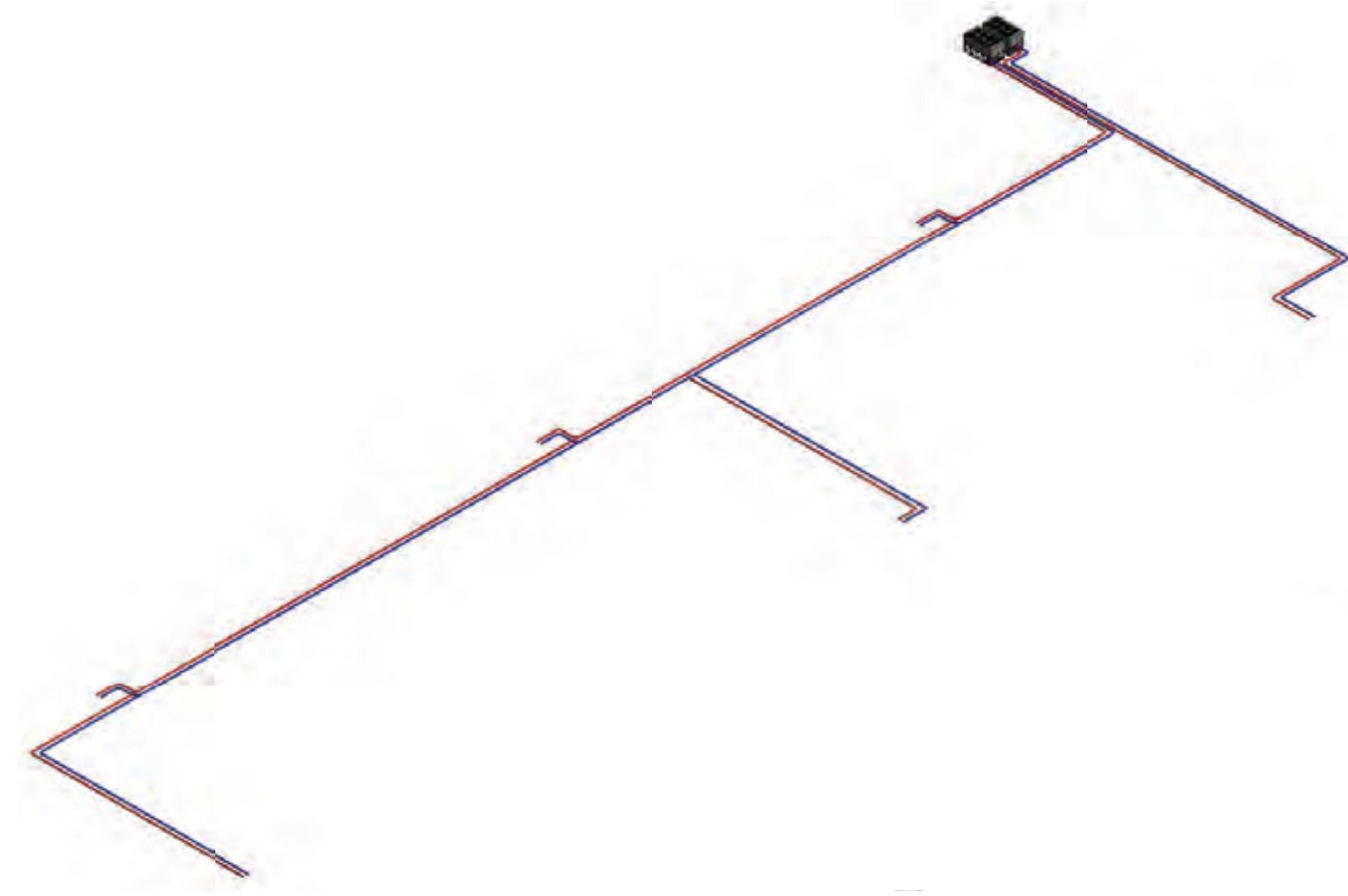
Chilled Water Piping for Air Conditioning
