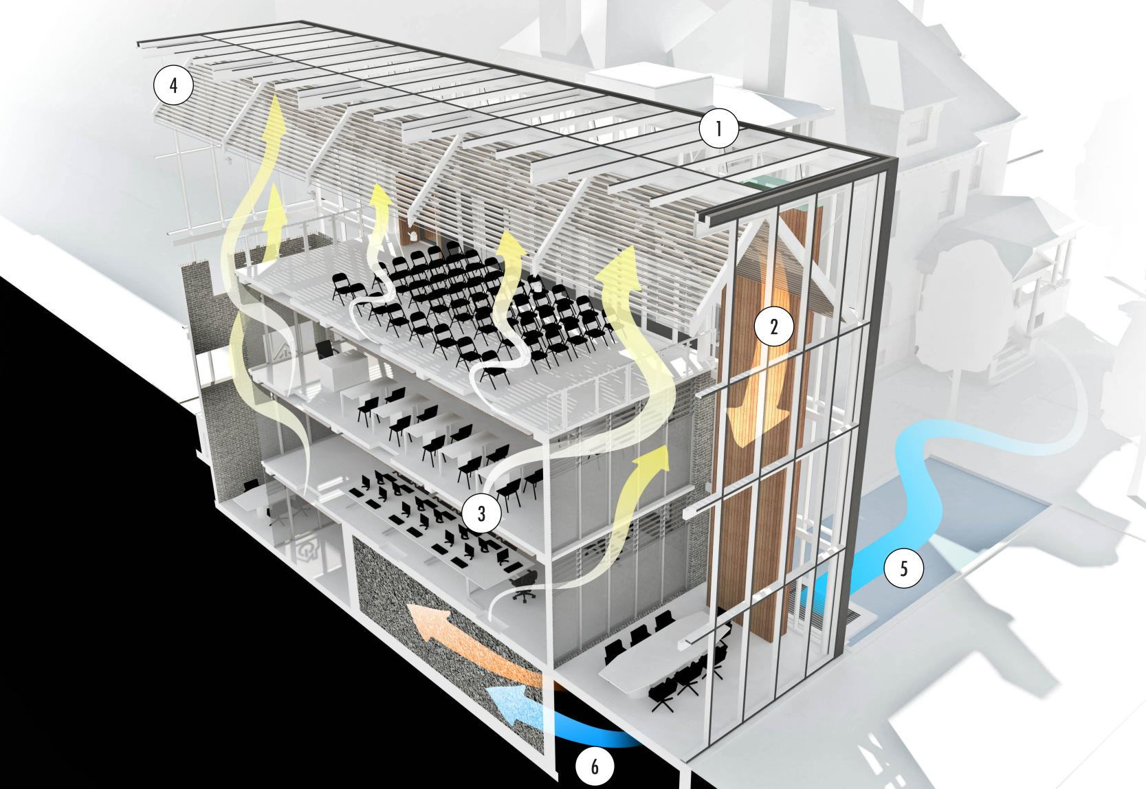
Solar radiation is trapped above pitched-roof louver system (1). Interior 'chimneys' pull hot air from the roof into a rock bed below the building (2). This heat is stored in the rock bed and released into the building above through the floors throughout the
