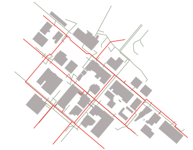
storm sewer + water system (red)
