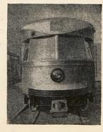
HE result of exhaustive wind-tunnel tests of conventional trolley car models revealed that at speeds of 70 and 80 miles per hour, 70 per cent of the total power was consumed in overcoming air resistance. Streamlining saves approximately 20 per cent of the power.
