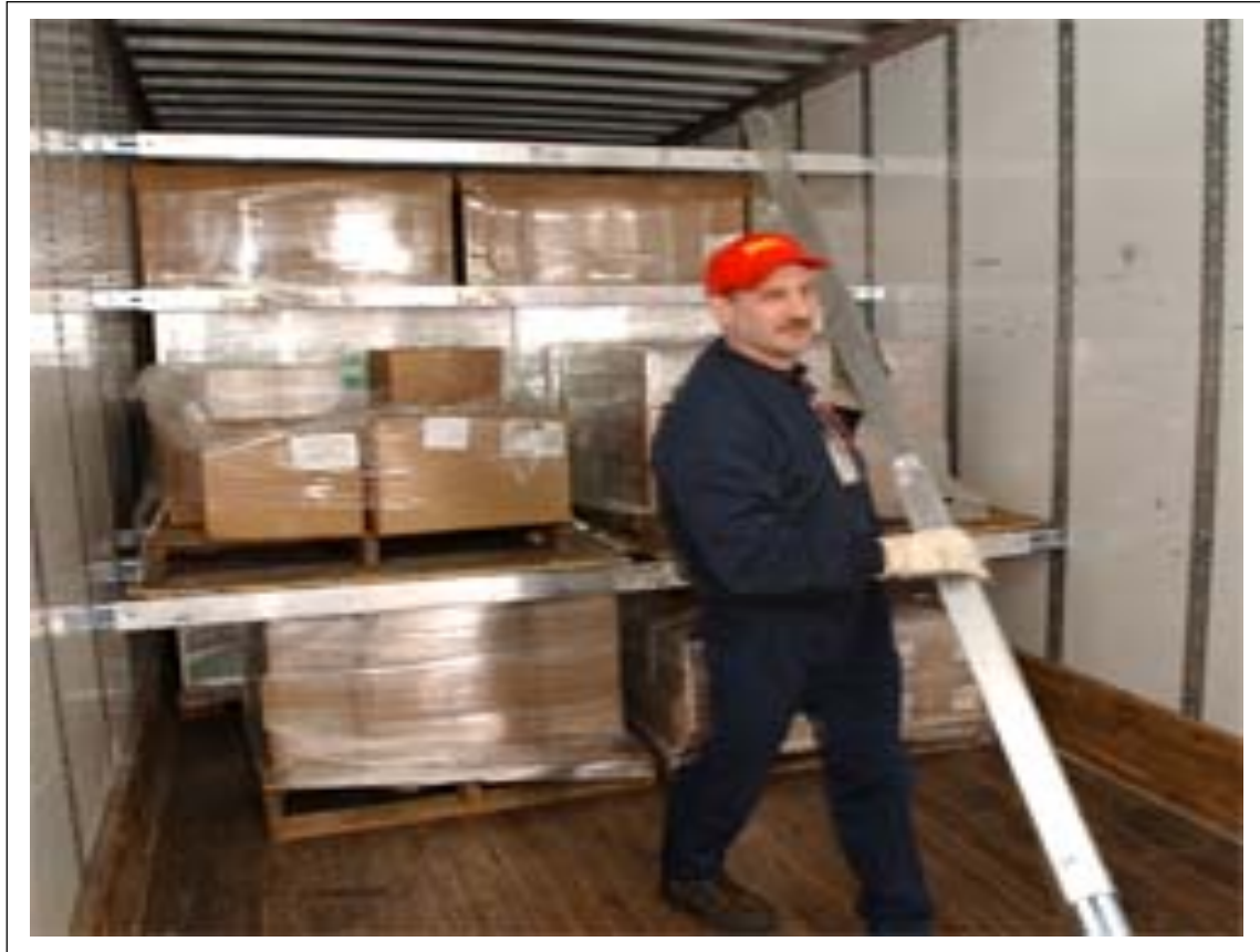
Figure 8. Picture of logistics beams in a trailer that can be adjusted to any height necessary and that can support up to 2,000 pounds in weight.
