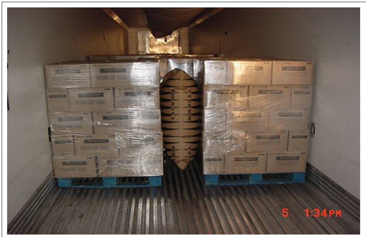
Figure 9. Picture of an air bag placed in a trailer at an HEB distribution center.
