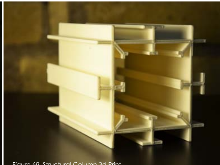
Figure 69. Structural Column 3d Print
