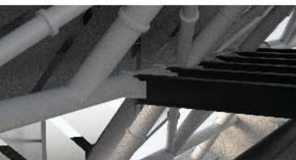
Level 2 Lateral Bracing
