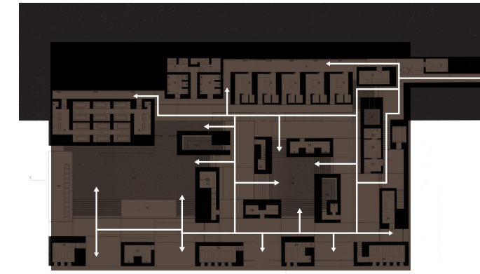
Circulation to use Thermevals bath (peter zumthor thermal vals, 2007) Figure.26. Thermal Vals Circulation to Use Diagram
