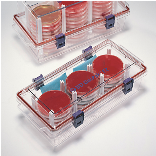
Figure 11. Becton, Dickinson and Company (BD) GasPak™ EZ Large Incubation Container. Used to produce atmospheres suitable for anaerobic, microaerophilic, or capnophilic bacterial growth. Gas generating sachets are placed inside the chamber, the chamber is sealed and the atmosphere is altered. In this study, the atmosphere inside the chamber was altered to allow anaerobic growth.
