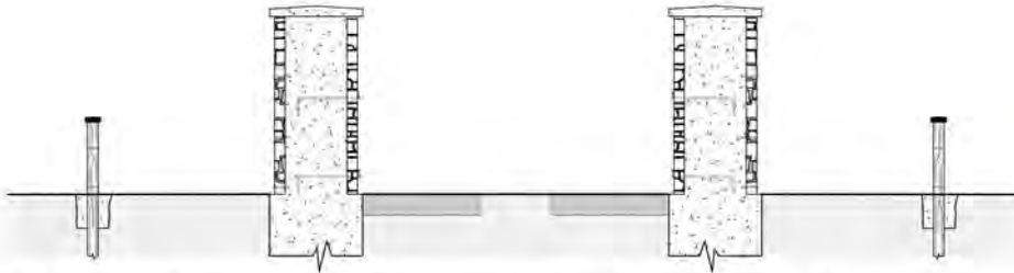
1. The gate's design includes two six-foot tall masonry pillars.
