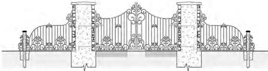
2. Each one filled with cement, would have appropriately scaled footings and would be used to support the gate's rod iron works.
