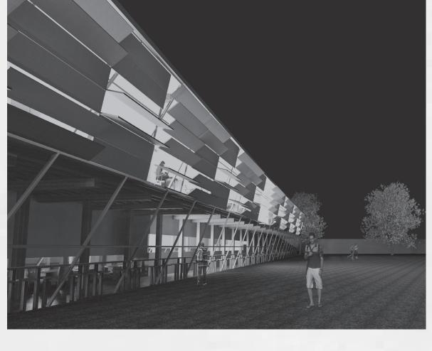
Exterior louvers are offset from the curtain wall to allow ambient light in even when closed. When open, the angles and size limit views from the ground.
