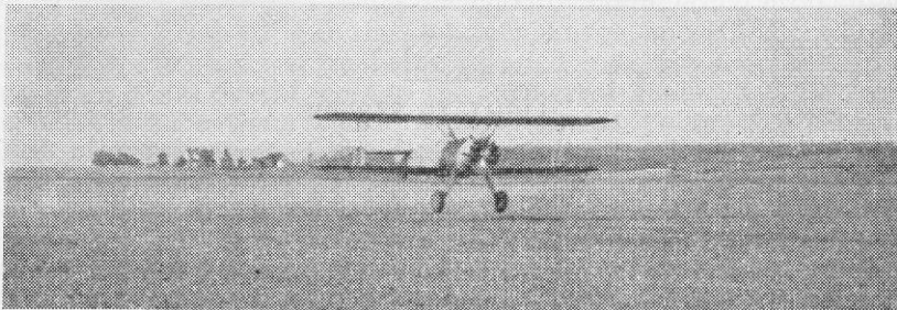
Fig. 3. Applying the spray in plane-width strips at the rate of about 75 miles per hour,—covering more than one acre per minute. Note the mist-like spray particles trailing behind.
