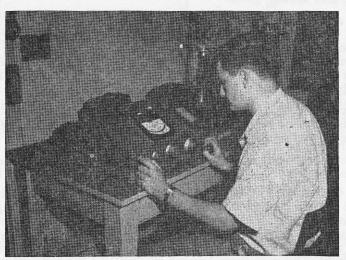
Final Test of any bread wheat is its mixing and baking quality, as determined by the cereal technologists. Here John Sullivan, student in chemical technology, at North Dakota Agricultural College, has determined the mixing requirements of a new hard red spring wheat hybrid to see if it conforms to accepted standards. Since mixing behavior is largely conditioned by the properties of the gluten, the student technologist seeks to learn the basic cause of gluten differences.
