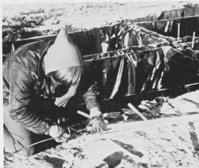
Figure 4. A system to allow drainage of unsaturated soil was constructed of porous cups and installed in each lysimeter.
