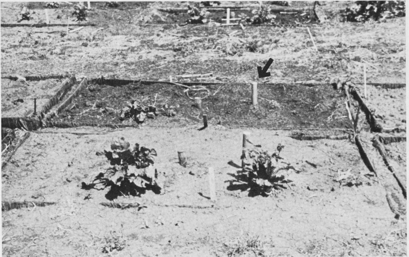
Figure 6. Lysimeters with growing sugarbeets. The arrow indicates the steel access tube for soil water monitoring equipment.
