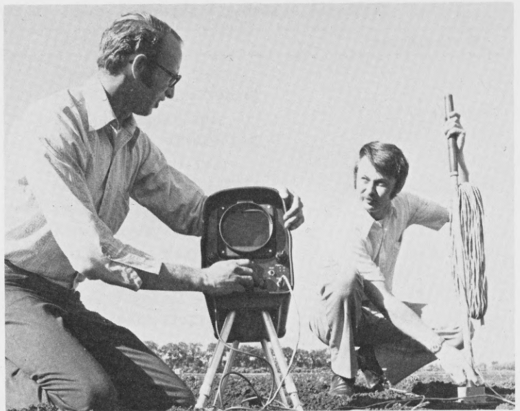
Dr. Bruce Worcester and Dr. Lynn Brun use a portable refraction seismograph to detect and measure the depth to subsurface layers important in measuring saline seep development.
