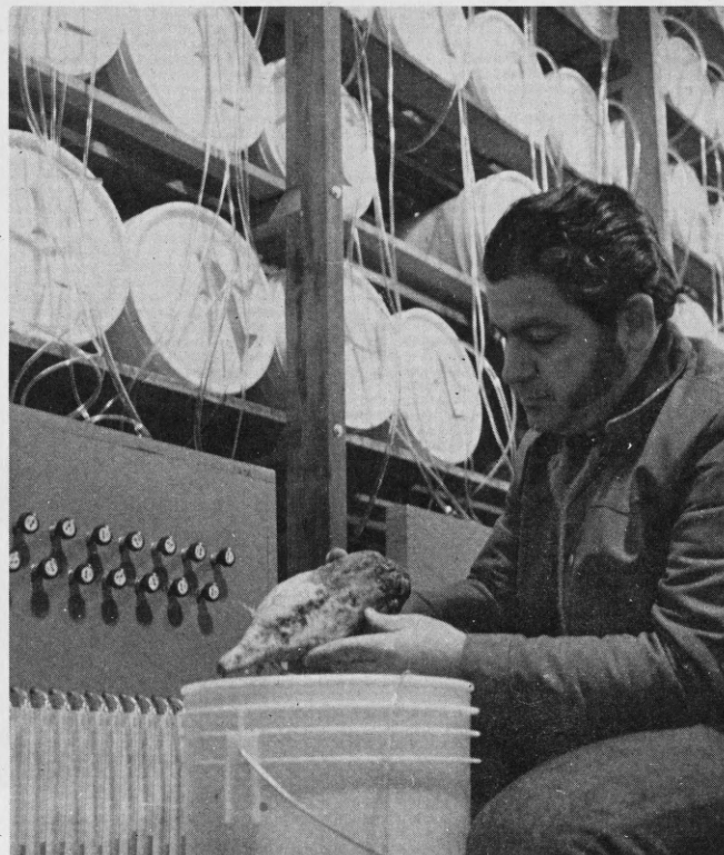
Dr. Darrell Cole, USDA-ARS plant physiologist at NDSU, measures the rate of respiration in sugar beets. Beets with slower respiration rates should lose less sugar during storage.
