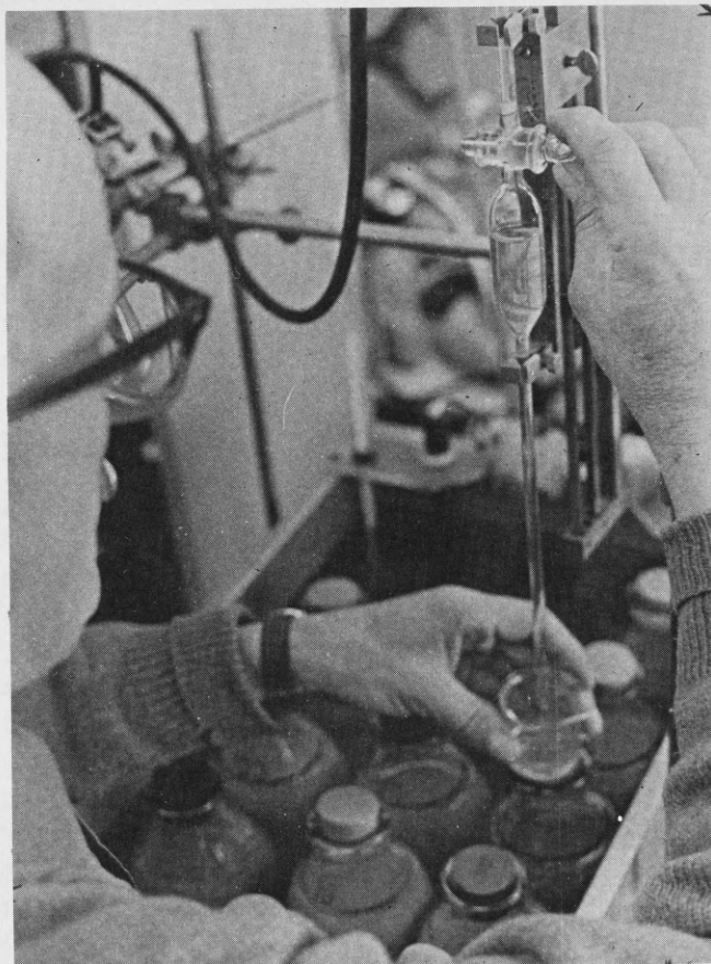
Particle size analysis is conducted on deep probe soil samples taken from an area with mining potential.
