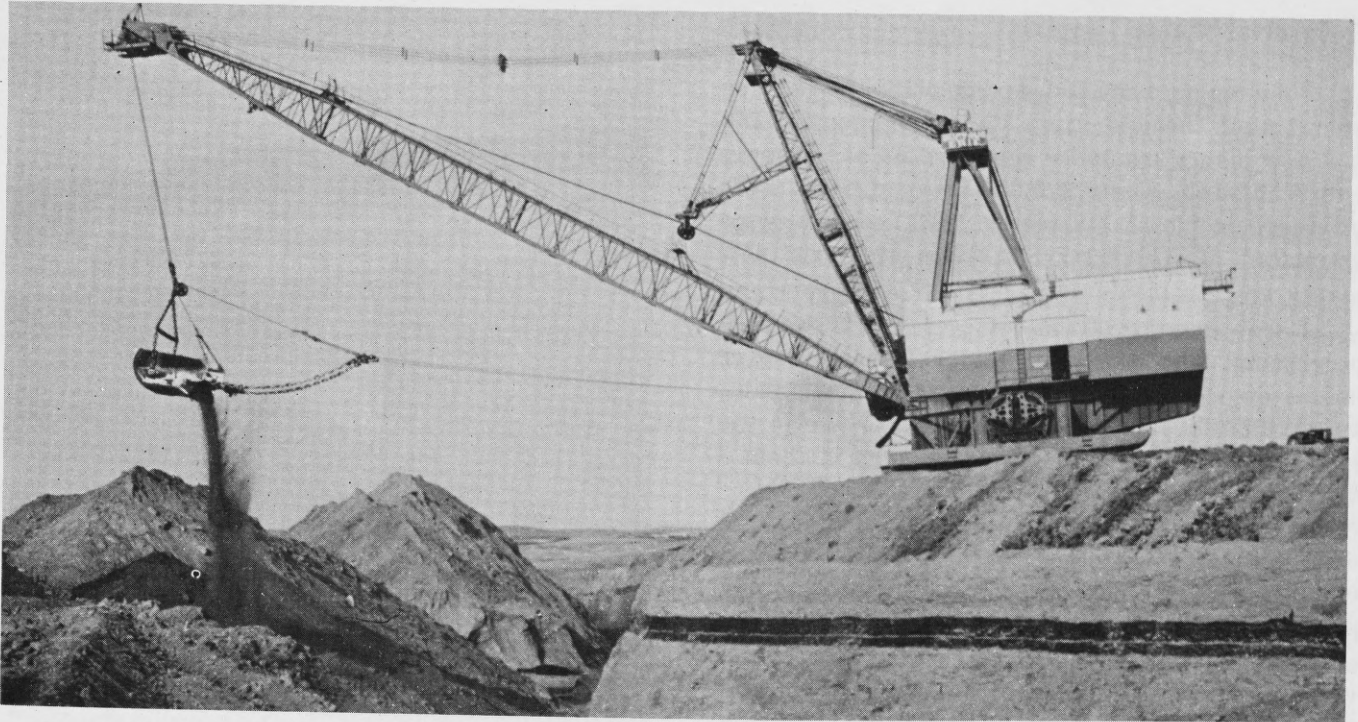
One of the unique features of the immense lignite coal reserves of the Fort Union Formation in western North Dakota is that it lies so close to the ground surface for economical strip mining operations. Strip mining, however, causes other environmental impacts that need to be studied and fully reported.
