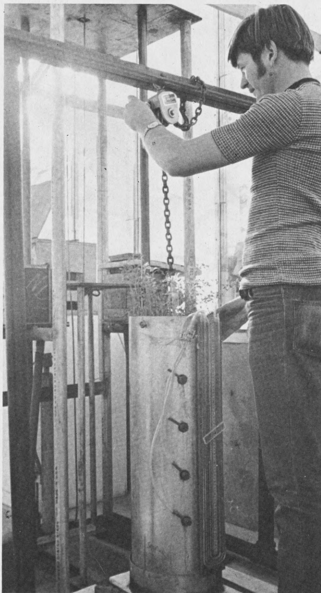
Figure 3. The hoist is used to lower the soil core onto a dolly, which is then pushed onto the movable carrier. The movable carrier is then elevated to the desired height(s) and the water content determined.
