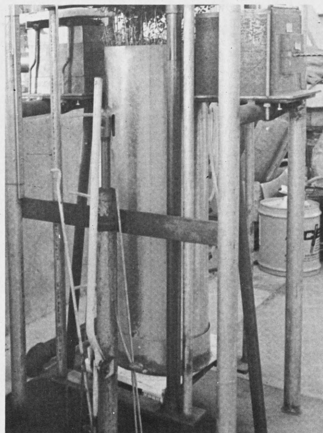
Figure 2. The proportion of gamma radiation emitted from the Cs 137 source housed in the center of the lead block passing through the soil core is detected by the scintillation detector. The radiation intensity is displayed on a scaler-timer. The hydraulic jack is used to elevate the movable carrier holding the soil core.
