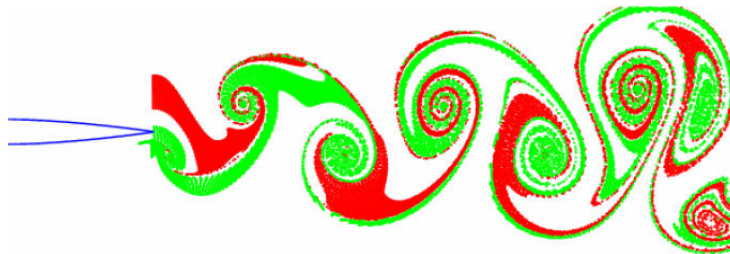
Figure 20: Trailing Edge Vortices [40]
