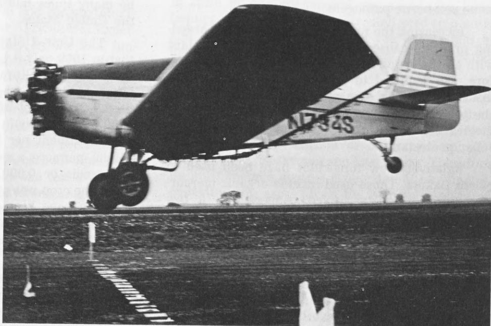
Spray pattern test for calibrating aerial application of liquid pesticides.
