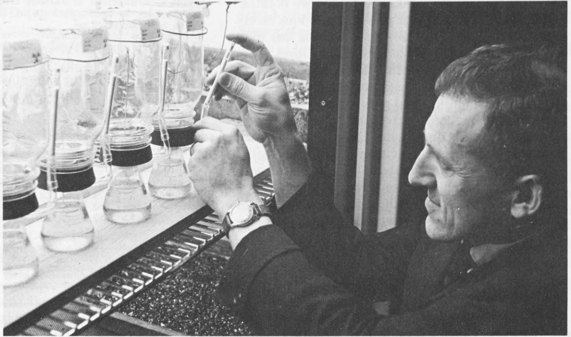
Dr. Nalewaja checks herbicide volatility from plants as influenced by spray solution additives.
