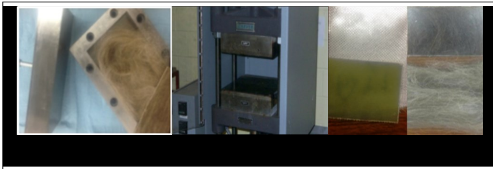
Figure 3-1. Scheme of the preparation of composite: (a) Mold prior to resin mixing, (b) Press machine, (c) Flax/MSSP and E-glass/MSSP composites.
