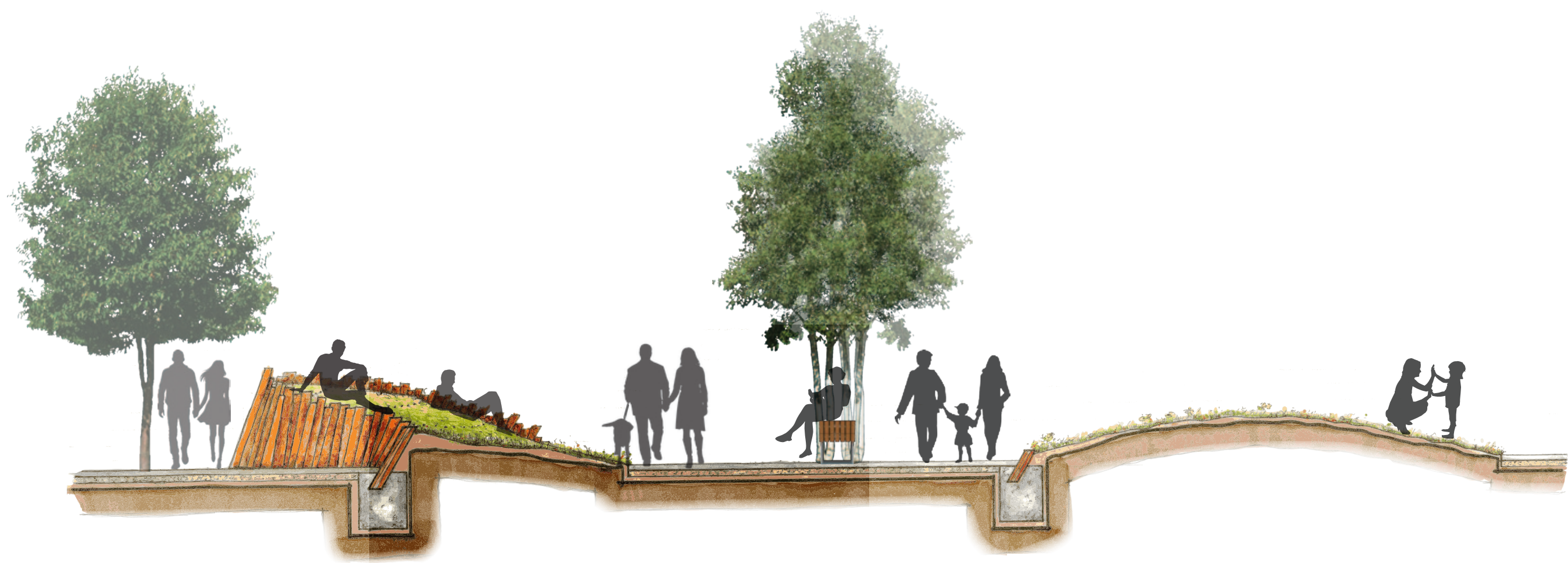
concrete walk | rail track retaining wall | 25'-00" concrete walk | rail track retaining wall
