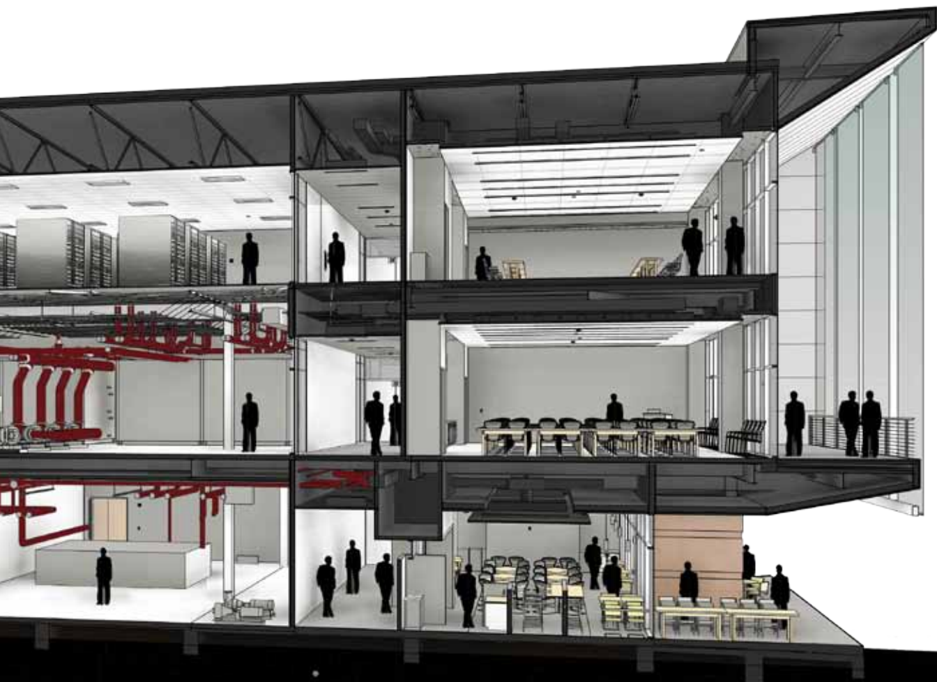
Figure 5.43 Server heating section. http://www.enterprisenetworkingplanet.com/datacenter/department-of-energy-using-warm-water-to-cool-data-center.html
