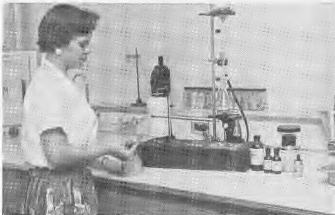
Fig. 2. Determination of the tenderness of cooked macaroni. The progress of breakdown of the macaroni piece is traced automatically on the paper in front of operator.
