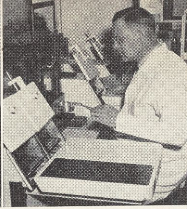
Butter samples are tested for percentage fat, water, salt and curd by Lyle Beck, NDAC analyst.
