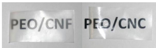
Figure 2.3. PEO/CNF and PEO/CNC nanocomposite films at room temperature. CNF and CNC concentration: 7%.
