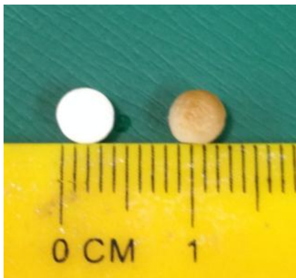
Figure18. Alginate-nZnO bead; freshly synthesized (left) and recovered (right) from treated liquid manure.
