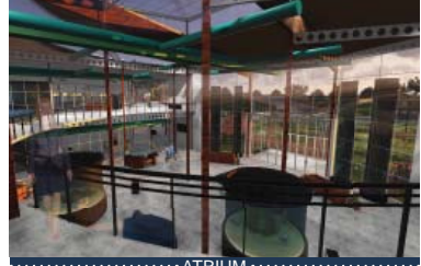
ATRIUM WITH CLERESTORIES AROUND THE PERIMETER, A LARGE SKYLIGHT IN THE CENTER, AND A SOUTH-FACING CURTAIN WALL, THE DOUBLE-HEIGHT ATRIUM IS AN INVITING GATHERING PLACE
