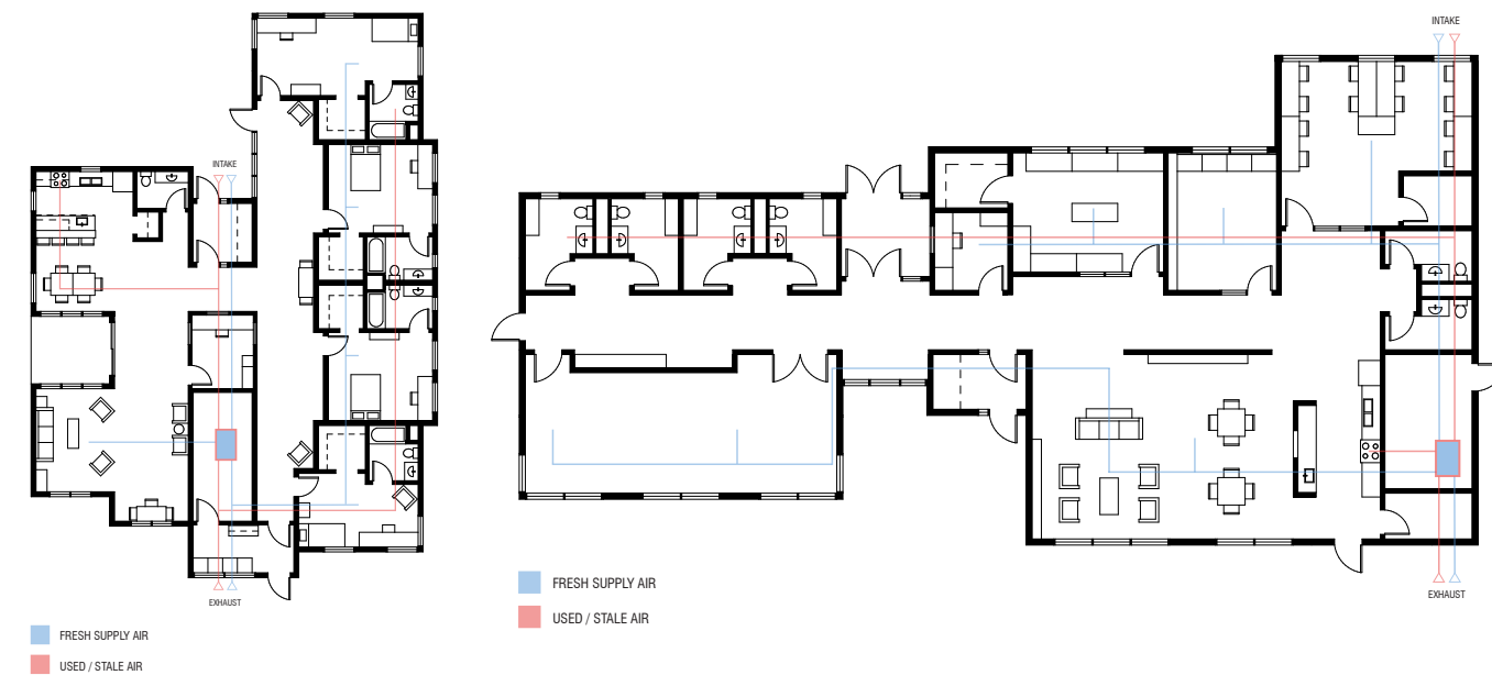
Figures 76 and 77 | Mechanical plans showcasing the proposed heat exchange system and function
