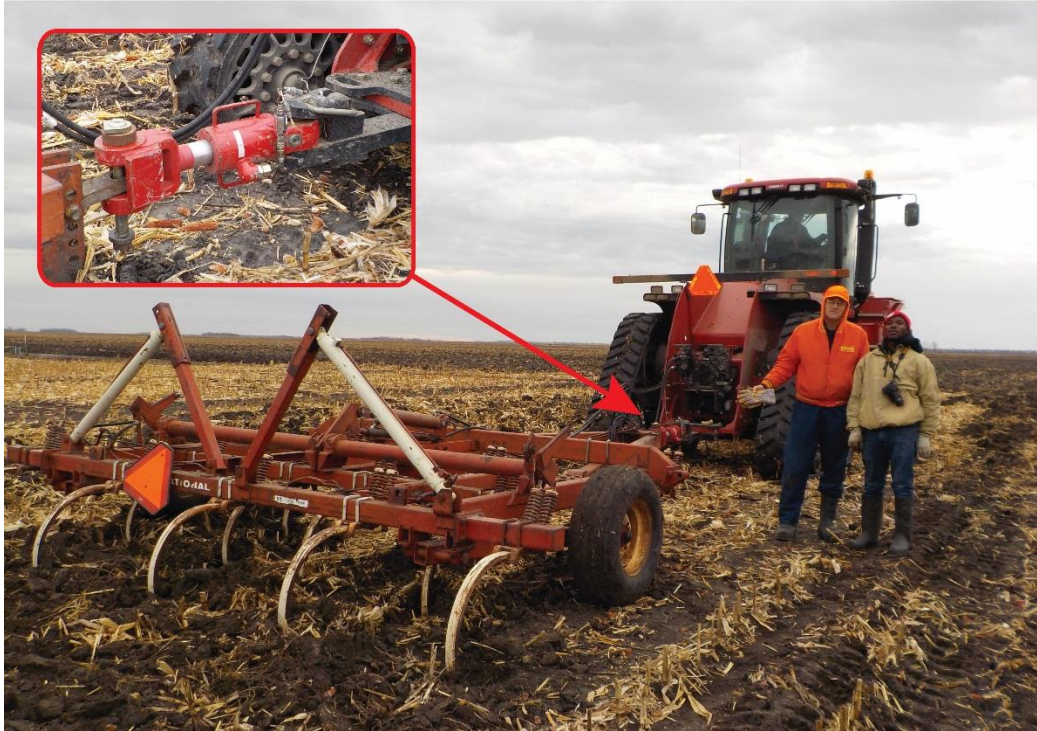
Figure 8. Tractor, pull meter, and chisel plow used to measure draft during tillage at an experimental field site near Wyndmere, North Dakota. The insert shows the pull meter used to measure draft on the chisel plow.
